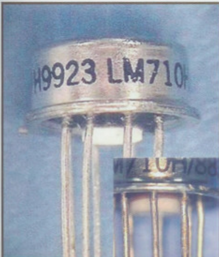
Figure 1: Note incorrect date code, incorrect header, and solder dewetting.
