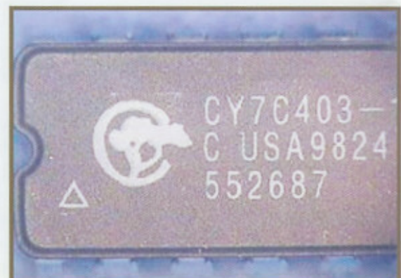
Figure 2: Note poor copy logo and suspect date code.
