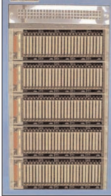
4000 test point CH2 mounted in a 19" rack
